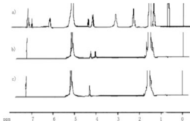
Figure 5 ^1\text{H} NMR spectra of (c) prepolymer E0%, (b) prepolymer E1%, and (a) prepolymer E1% coupled with TDI with OH/NCO ratio of 1:1.2.
